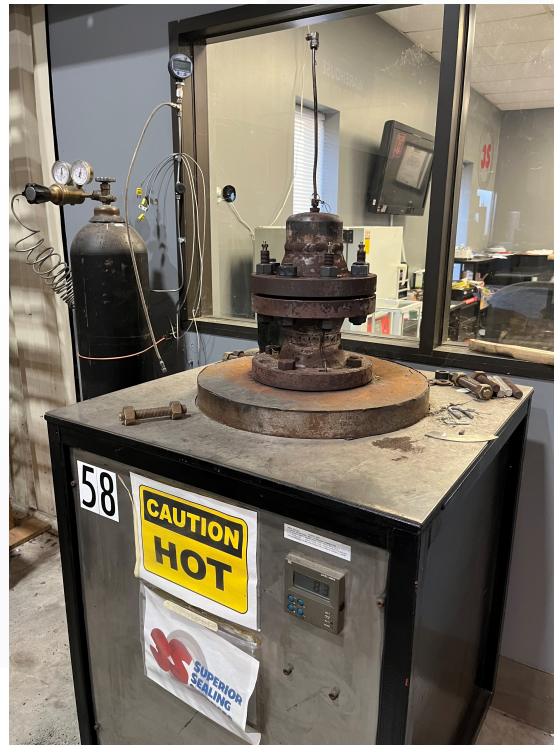
4" 300lb RF WN Flanges to ASME B16.5
