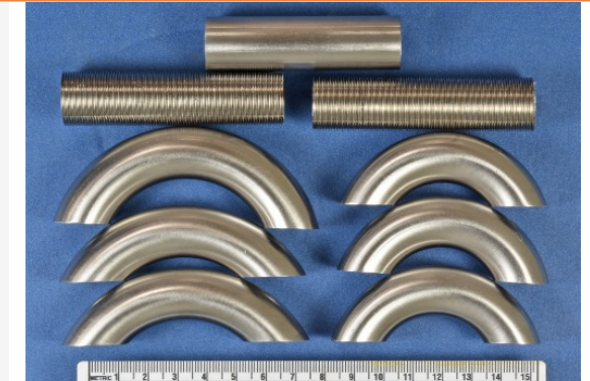
S32750 finned and u-bend samples bent to 1.5D and 2D shown on the right.
